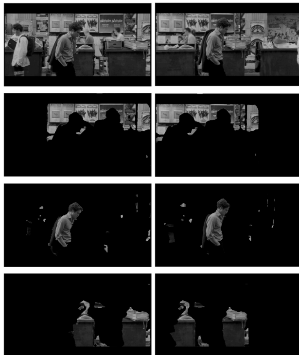
Figure 5: Notting Hill sequence. (1) Original image pair of size 311 \times 552 , (2-4) Pixels assigned to warp layers 1-3 in I and I' .
