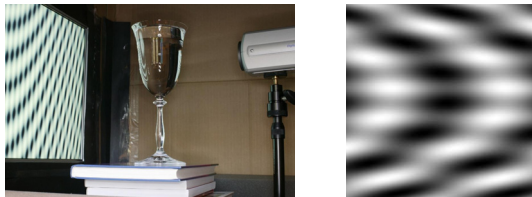
Fig. 2. (a) Shown above is a photograph of the data acquisition system used in our experiments. It consists of Samsung 19" LCD display screen on the left, a Sony DFW-VL500 firewire camera on the right and a refracting object between the screen and the camera. (b) shows a frame from the background image sequence for all our experiments.
