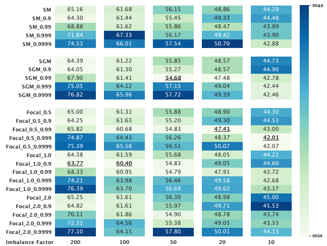
Figure 10. Classification error rates of ResNet-32 models trained with different loss functions on long-tailed CIFAR-100.
