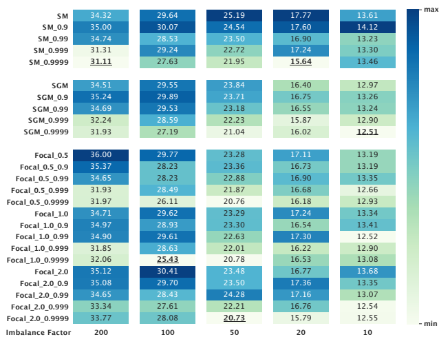
Figure 8. Classification error rates of ResNet-32 models trained with different loss functions on long-tailed CIFAR-10.
